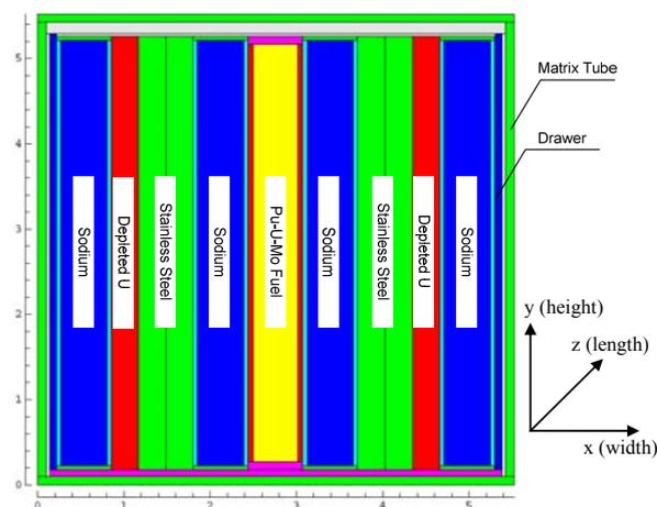
Fig. 1. Schematics of representative unit cell [cm]
