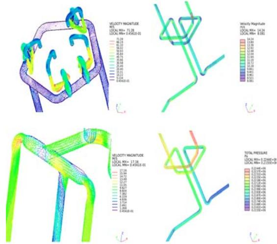
Fig. 5. Velocity magnitude and pressure distribution according to elevations of pipe line
