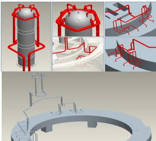
Fig. 1. 3D CAD domain for pipe line from POSRV to IRWST
