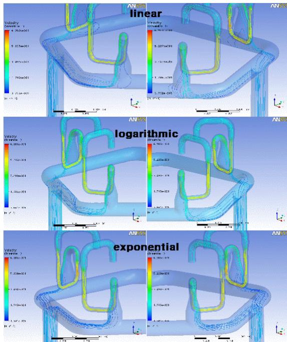
Fig. 4. Stream line according to POSRV operating condition
