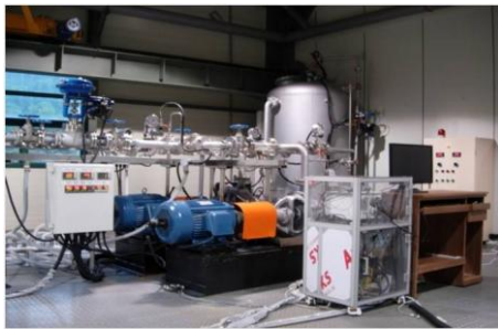
Fig. 1 Experimental apparatus for pump cavitation test
