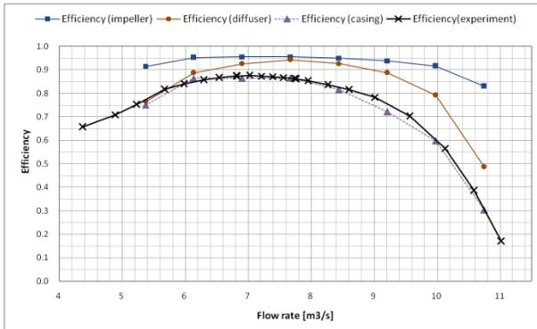
Fig. 2 Performance curves: efficiency.
