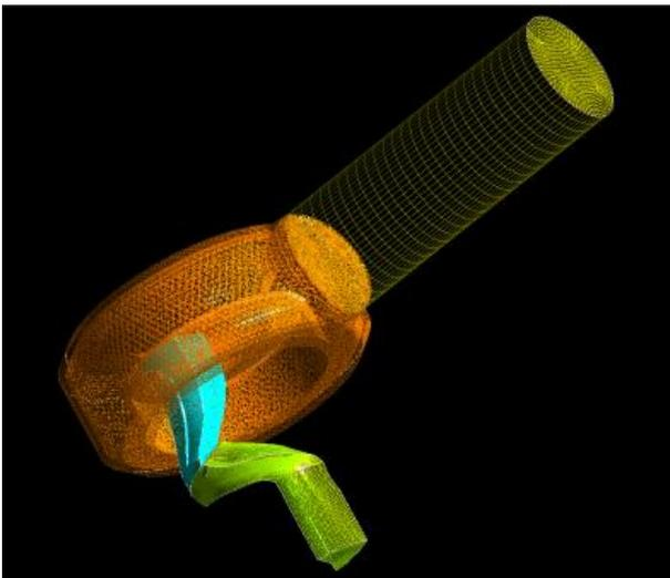
Fig. 1 Shape and the structure of grid systems of the RCP assembly.
