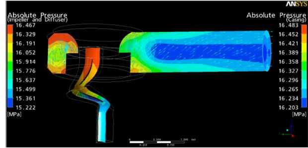
Fig. 4 Absolute pressure distribution on virtual planes in the RCP
