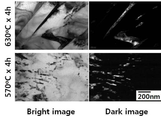
Fig. 4 TEM micrographs of the HANA-4 alloy annealed at 570 °C and 630 °C for 4h
