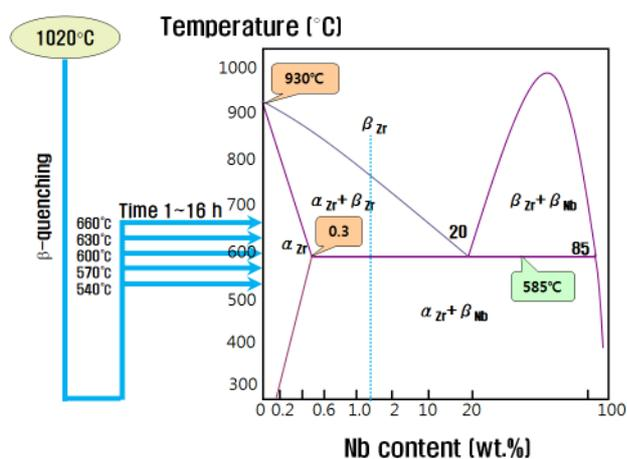
Fig. 1 Schematic illustration of annealing conditions of HANA-4 (Zr-1.5Nb-0.4Sn-0.2Fe-0.1Cr) alloy after  $\beta$ -quenching
