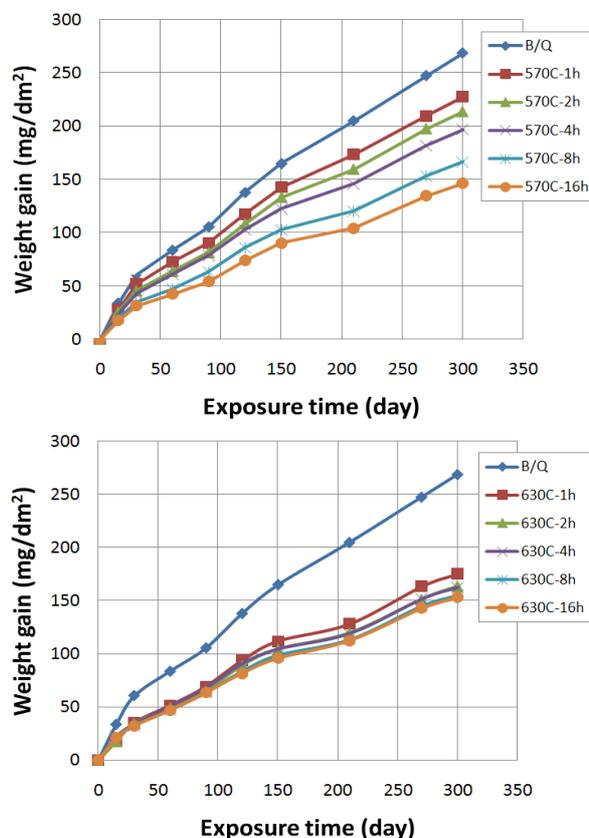
Fig. 2 Corrosion behavior of HANA-4 alloy annealed at 570 °C (upper) and 630 °C (lower) after  $\beta$ -quenching
