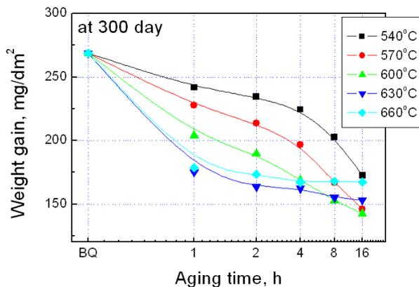
Fig. 3 Comparison of corrosion weight gain with the annealing time and temperatures of HANA-4 alloy
