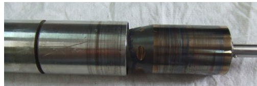
Fig. 4 Magnet separation from the shaft
