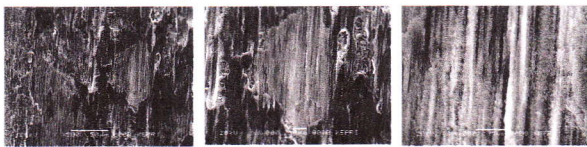
Fig. 5. Worn surface of alloy 690 against flexible gasket (P-1)
