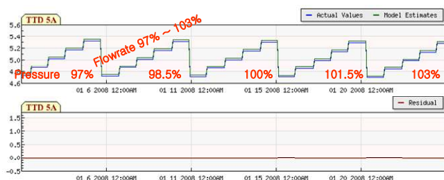
Fig. 2 Leak monitoring program results for normal condition in TTD5A (feedwater flowrate: 97%~103%, main steam pressure: 97%~103%)
