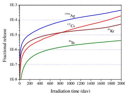
Fig. 3. Fractional release evolution of fission products into a coolant.
