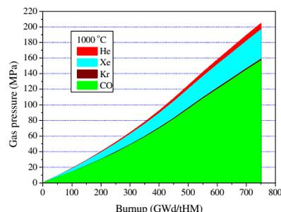
Fig. 1. Gas evolution in the buffer of a CFP.
