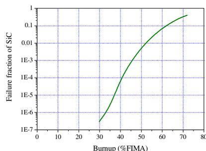
Fig. 2. Failure fraction of SiC when the number of Monte Carlo runs is  $10^7$ .
