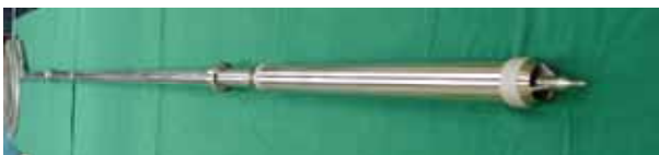
Fig. 1. An Instrumented Fuel Capsule
