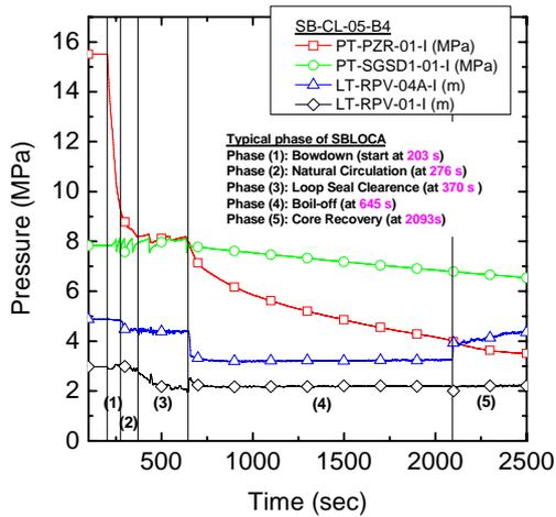
Fig. 1 Cold leg SBLOCA characteristic phase separation of SB-CL-05
