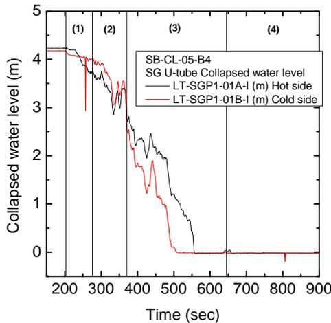
Fig. 2 Collapsed water levels in the SG U-tube in case of SB-CL-05
