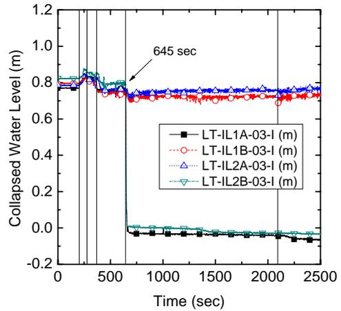
Fig. 3 Cold leg SBLOCA characteristic phase separation of the SB-CL-05
