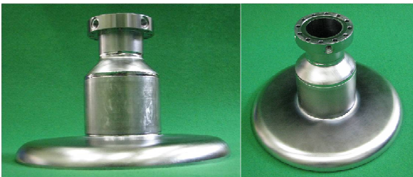
Figure 4. End cell sub assembly. Left: FPC beam tube. Right: Field probe beam tube.
