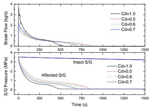
Figure 2. Break flow and S/G pressure
