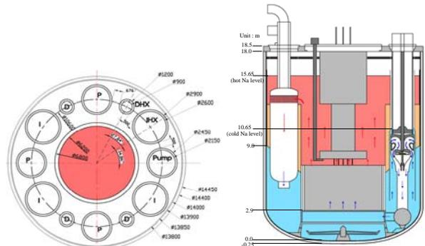
Fig. 2. Component arrangement for 1,200MWe pool-type burner reactor.
