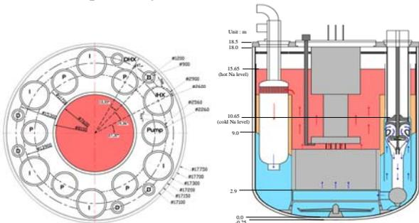
Fig. 3. Component arrangement for 1,800MWe pool-type burner reactor.
