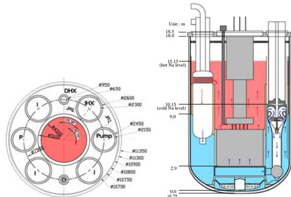
Fig. 1. Component arrangement for 600MWe pool-type burner reactor.
