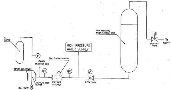
Fig. 2. Schematic of test system at reverse flow
