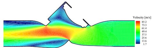
Fig. 5. Velocity contour within the valve operating at supply velocity 10m/sec
