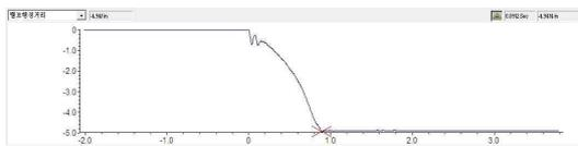
Fig. 4. Valve disk position during the reverse flow
