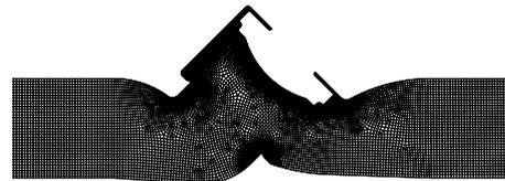
Fig. 3. Computational meshes inside valve
