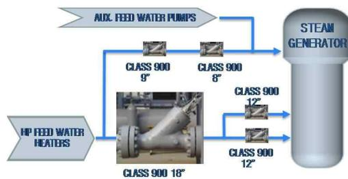
Fig. 1. Check valve mounted on the line in nuclear power plant
