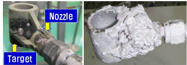
Figure 5 Assembly image of after a Na-H 2 O (left) and Na-CO 2 (right) reaction
